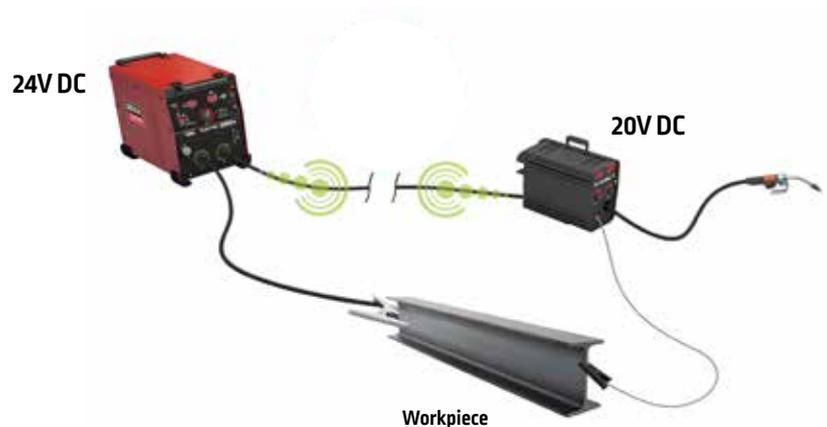
True Voltage Technology (TVT) sees this drop and gives you the true voltage you set by adjusting the power source to compensate for the voltage drop. In the example below, 24v is preset at the Activ8X wire feeder. TVT senses there is a 4 volt drop due to long weld cables and compensates by increasing the welder output to 28V. The result is the desired 24v available at the welding arc.
