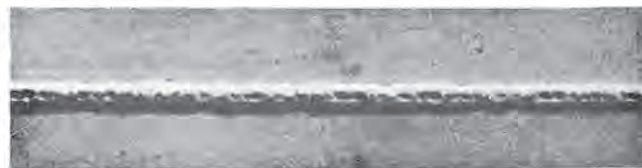
FIGURE 5 — Porosity caused by oily plate.
