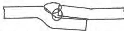
FIGURE 11 — Offset-lap welds inherently tend to trap flux in the bottom of the joint. First pass may be porous; second pass is sound.
