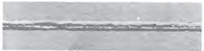
FIGURE 8 — Porosity from backward arc blow is more common on the finish end of welds in light gauge sheet metal than in any other type of weld.
