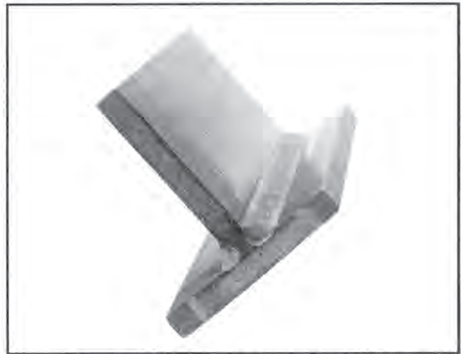
1/2" (12 mm) flat fillet welded at 540 amps at 15 in./min (0.38 m/min) with 3-1/4" (82 mm) stickout using a hand-held gun.
