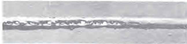
FIGURE 6 — Dirty flux can cause severe porosity.
